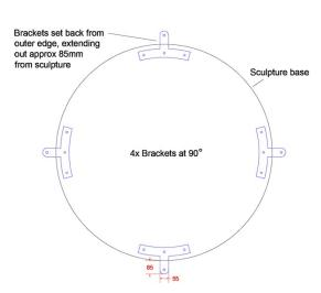
The globe sculpture (see separate document for specifications) will have 4 x metal brackets attached into 4 recesses on the base.
