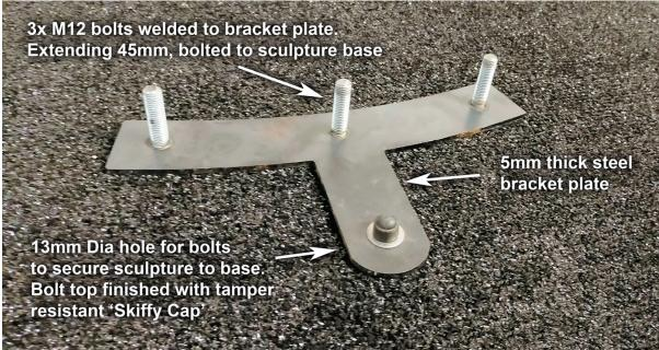
The top of the plinth will be made from 24mm marine plywood and the sculpture will be attached by bolting the 4 x bracket of as per below:
