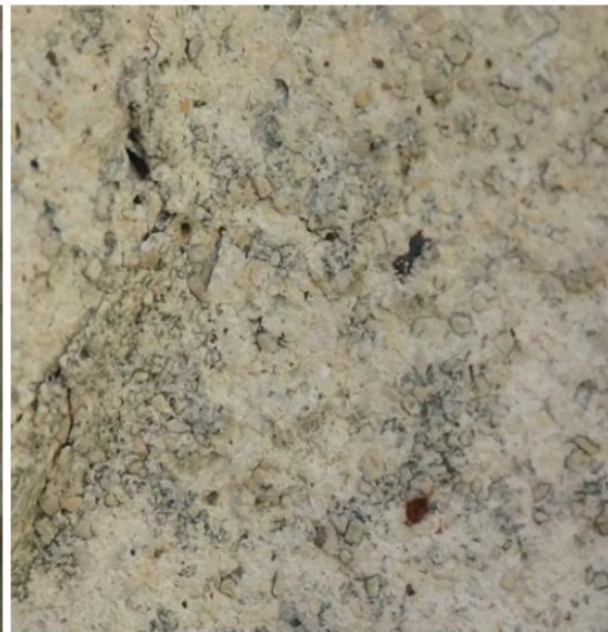
Figure 12 M3S.2. Drapery: Large particles of different colours and sizes. Note the dark red particles. Other areas show a sandier looking matrix.
