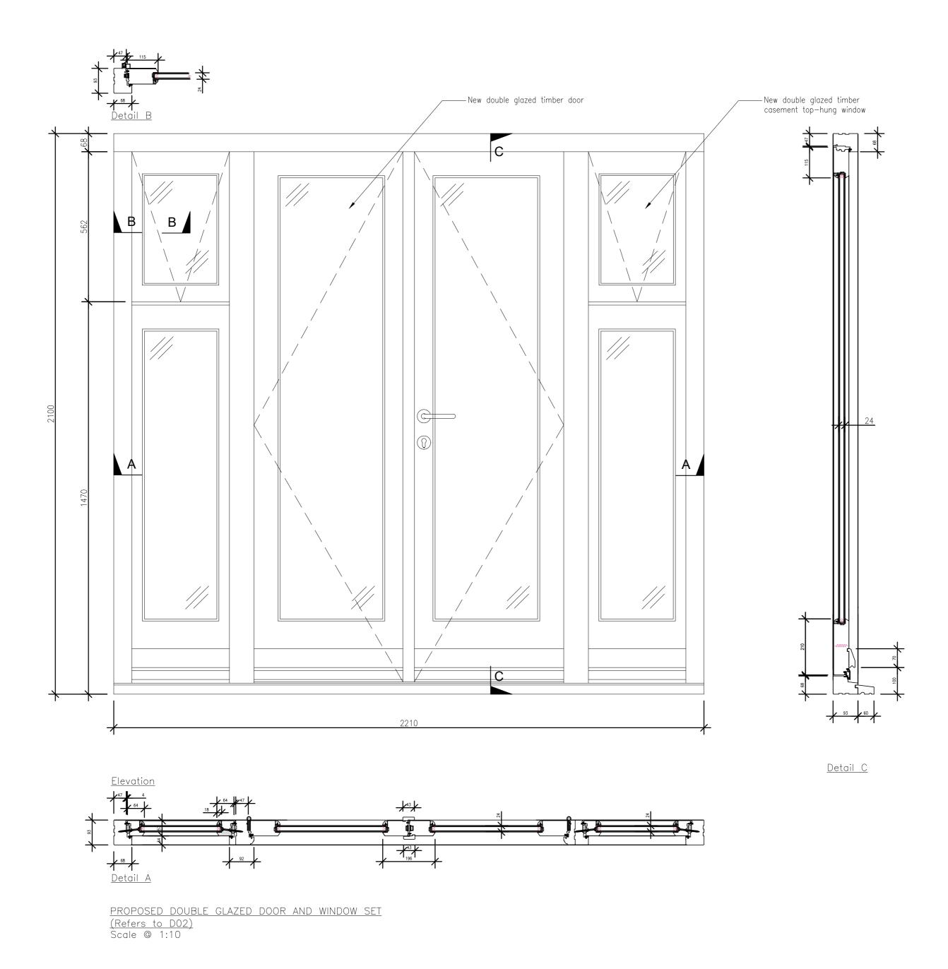
ALL DIMENSIONS, LEVELS AND CLEARANCES TO BE CHECKED ON SITE PRIOR TO WORKS COMMENCING
