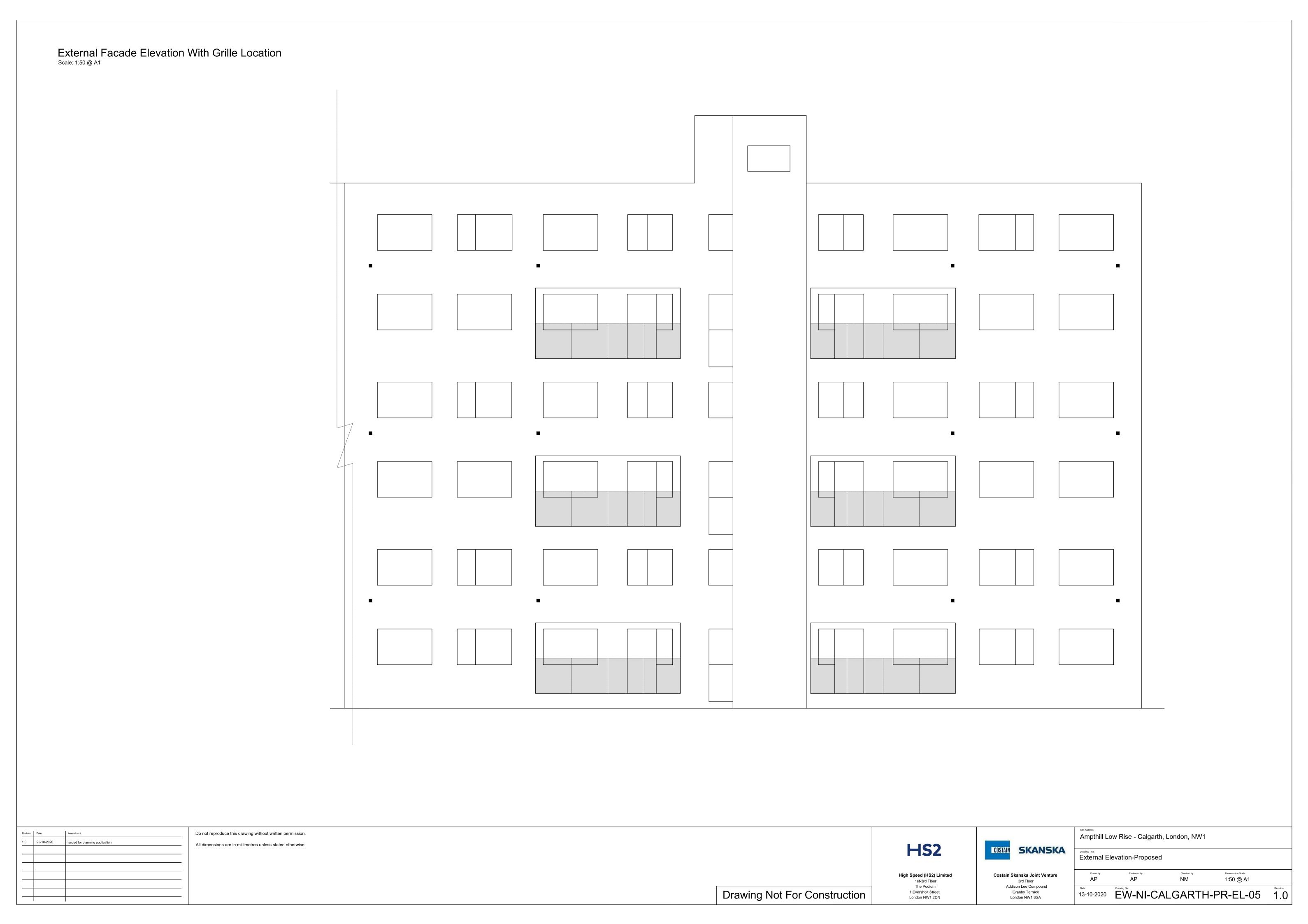
External Facade Elevation With Grille Location
