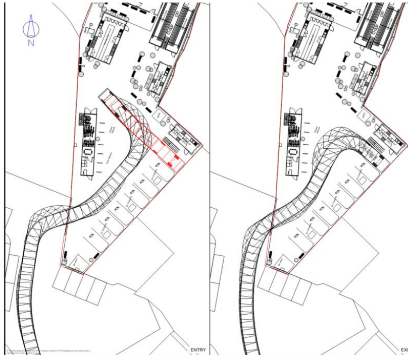
Figure 4. Swept path analysis of entry and exit
