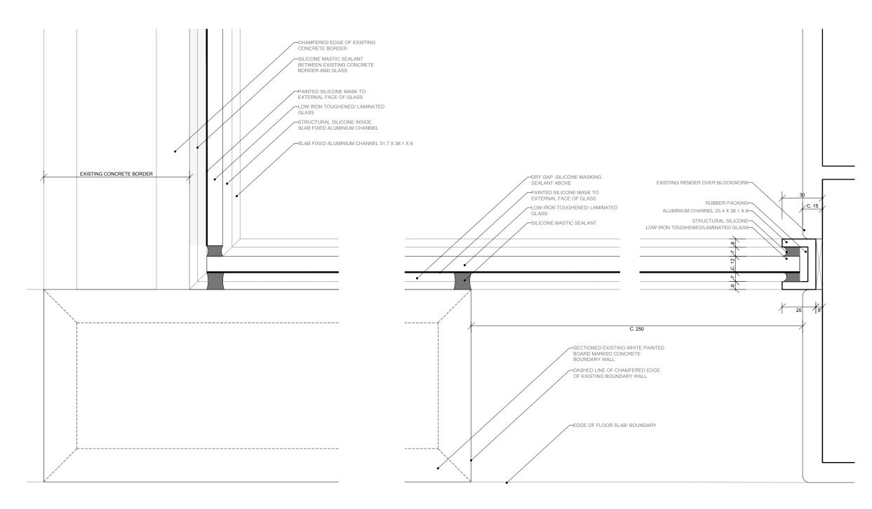
**DETAIL 1.1** Perimeter detail to existing low border wall (plan) **DETAIL 3.1** Glass to top of existing boundary wall (section)
