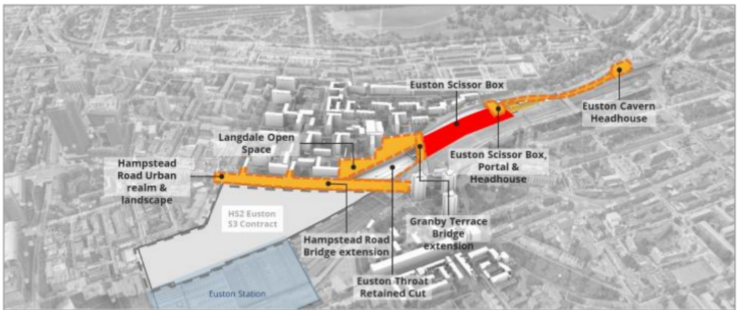
2. Proposed Scissor Box Roof Slab (in Red) and its surroundings
