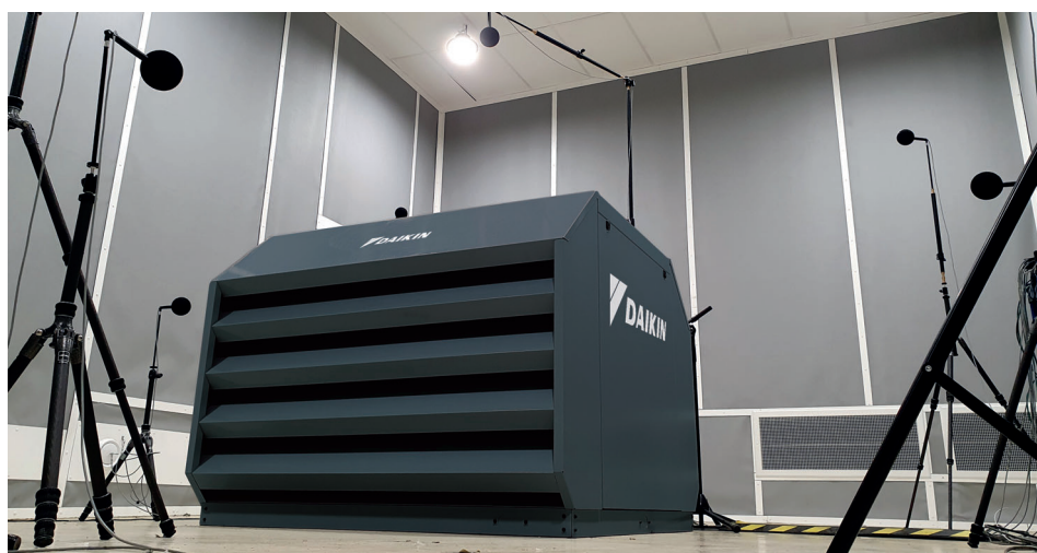
Sound power level measurement in acoustic chamber
