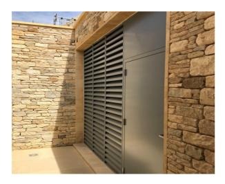
EMTEC LAAC 15-105 Acoustic Louvres can be installed as individual units or by bolting more than one unit together (horizontally or vertically) openings of any size can be accommodated. Each louvre has a robust outer framework which acts as vertical mullions and horizontal transoms when several units are fixed together. If a continuous blade effect is preferred this can also be supplied.
