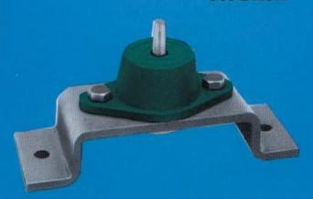
Thru bolt makes mounting and supported equipment captive. It prevents failure of mounting due to excessive horizontal and vertical shock. Recommended for shipboard and vehicular installations, or engine installations with high starting torque.
