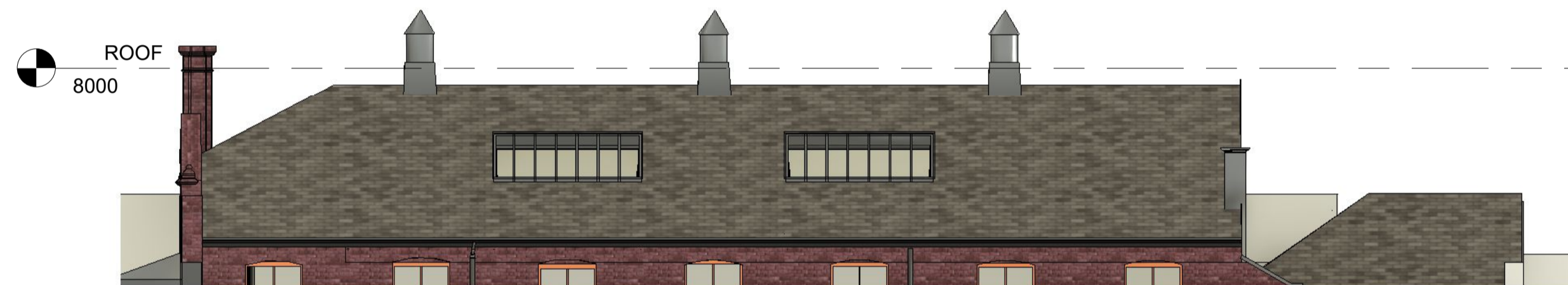
B EXISTING ROOF LIGHTS ELEVATION B 711 1:100
