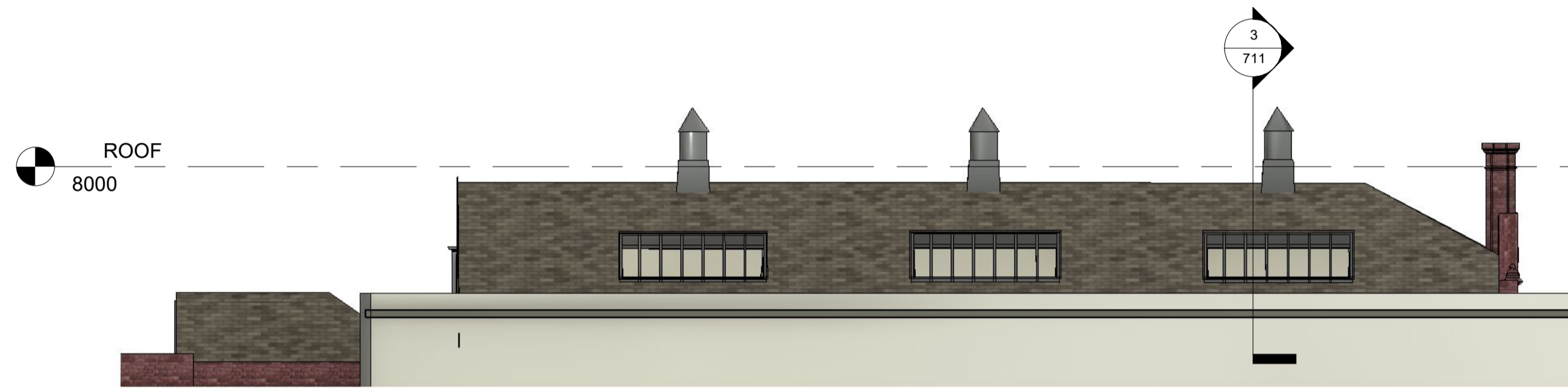
A EXISTING ROOFLIGHTS ELEVATION A 711 1:100
