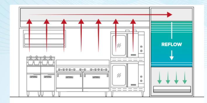
Extracted air passes through either 5 or 8 stages of filtration.
