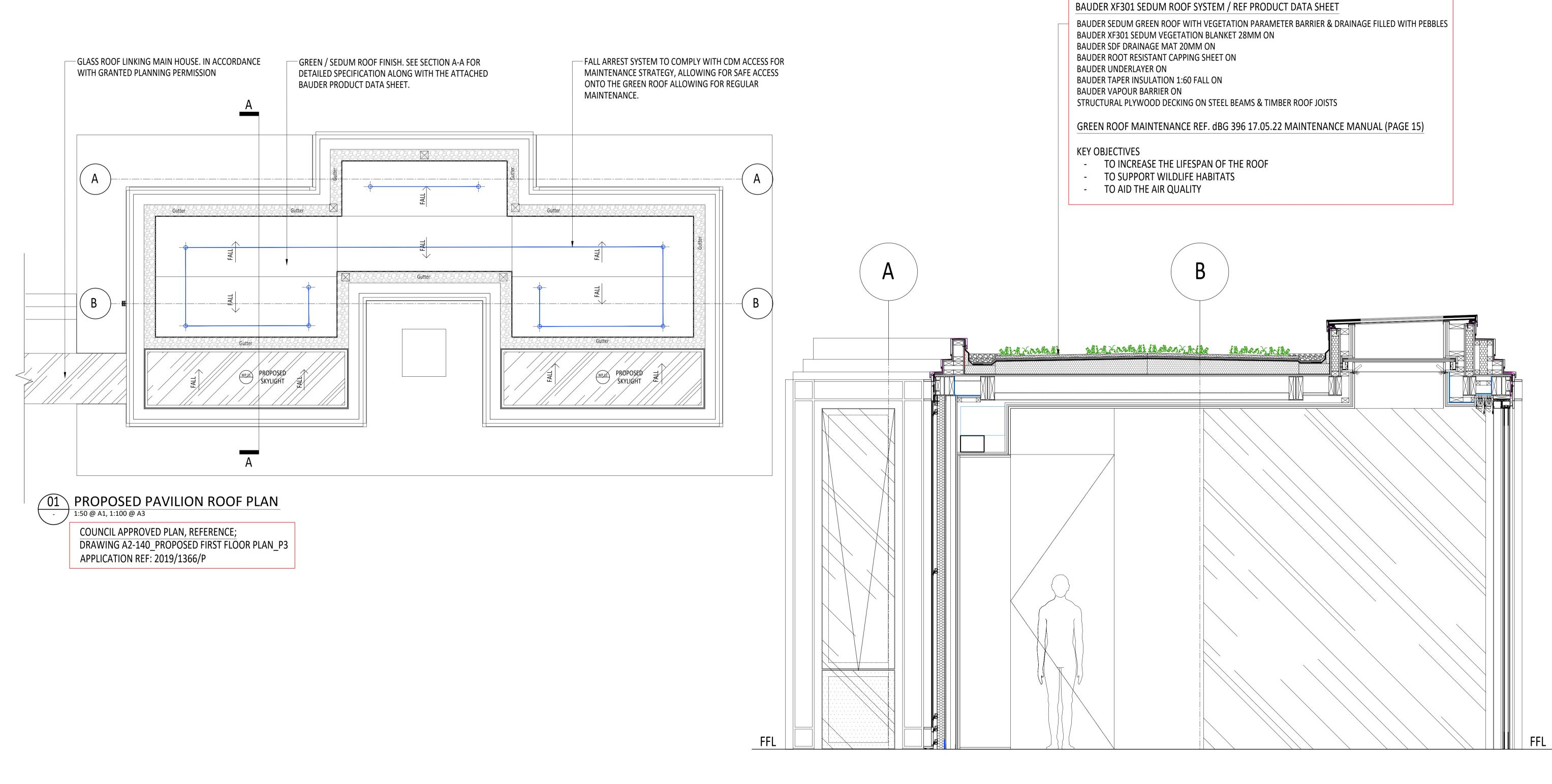
PROPOSED GREEN ROOF SECTION A-A 1:20 @ A1, 1:40 @ A3
