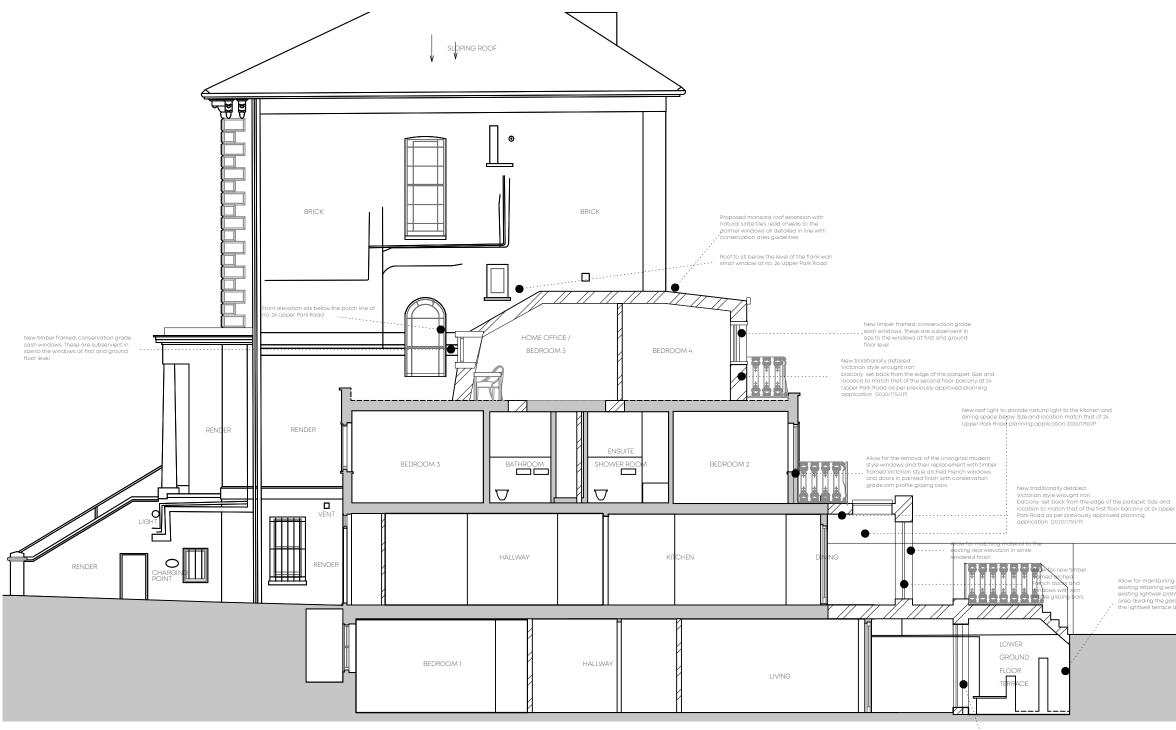
Allow for new timber framed double glazed windows and doors with conservation grade slim profile glazing bars in painted finish
