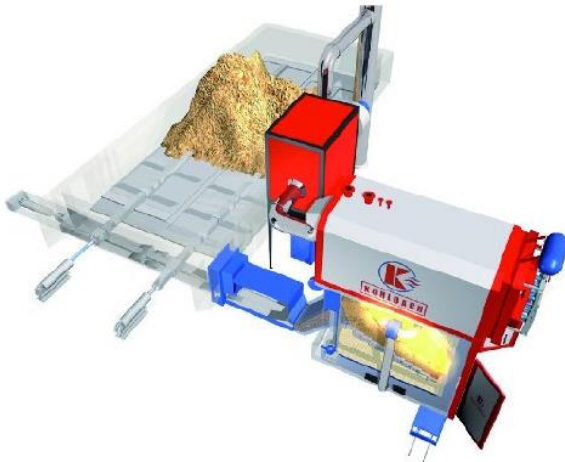
Figure 12 Typical Biomass Boiler and Auger © BSRIA.
