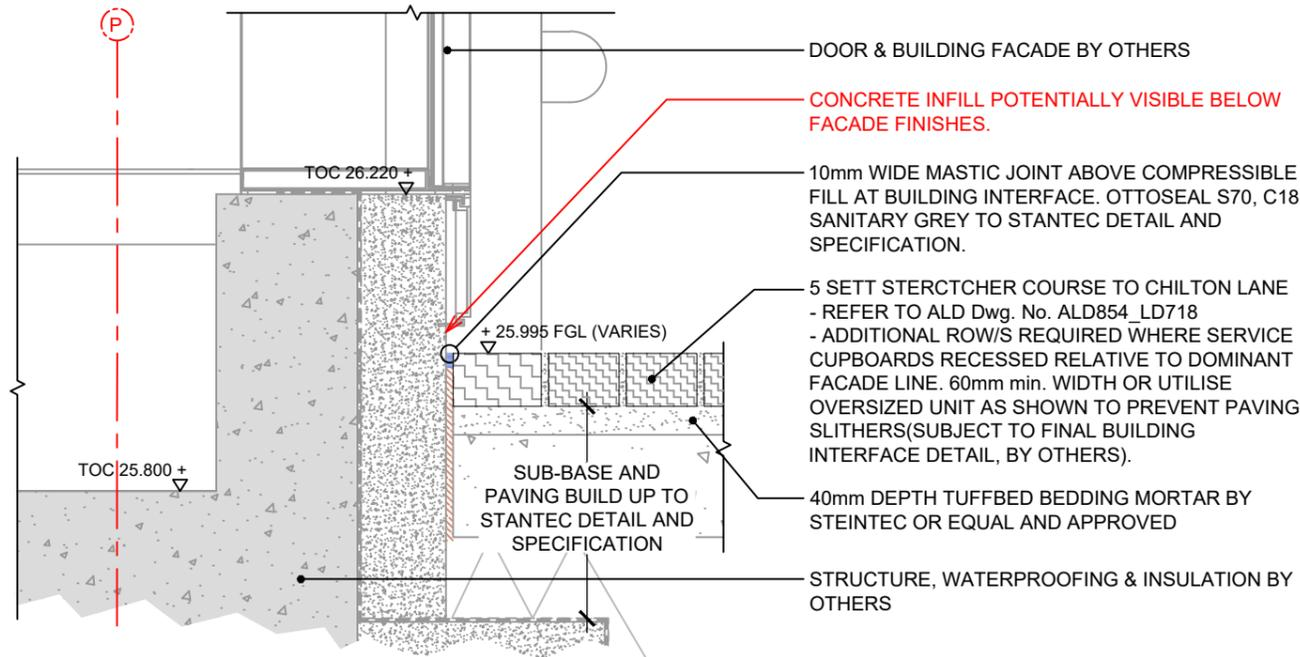
**32c** SECTION THROUGH GAS METER ROOM METAL DOOR INTERFACE WITH YORKSTONE SETTS TYPE 2
