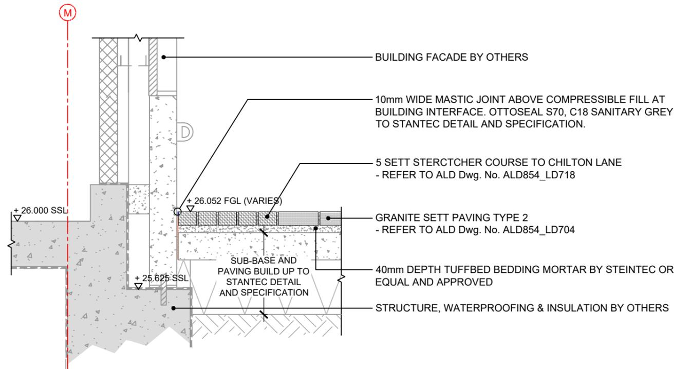
**32d** SECTION THROUGH PRECAST CONCRETE SKIRTING INTERFACE WITH GRANITE SETTS TYPE 2, CHILTON LANE
