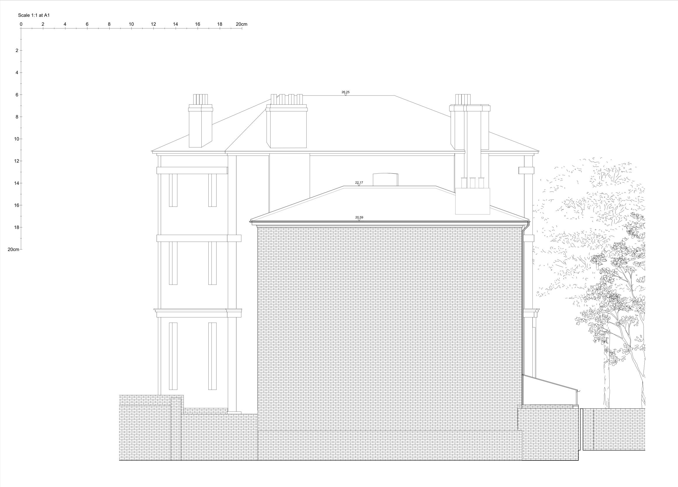
$01 \stackrel{\text{EXISTING SOUTH EAST ELEVATION}}{\scriptstyle 1:50 @ \text{A1}}$
