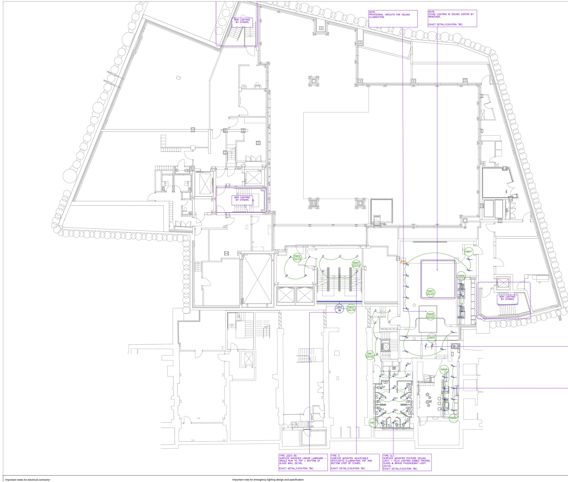
All directional light fittings to be angled by electrical contractor onto product/ displays/ artwork/ tables/ other in accordance with the lighting drawing/ any designer or client instructions. This must be carried out in advance of the final lighting commissioning/ any programming visit by the lighting consultant/ dimming engineer. Into Lighting do not carry out any works at high lovel. level.
