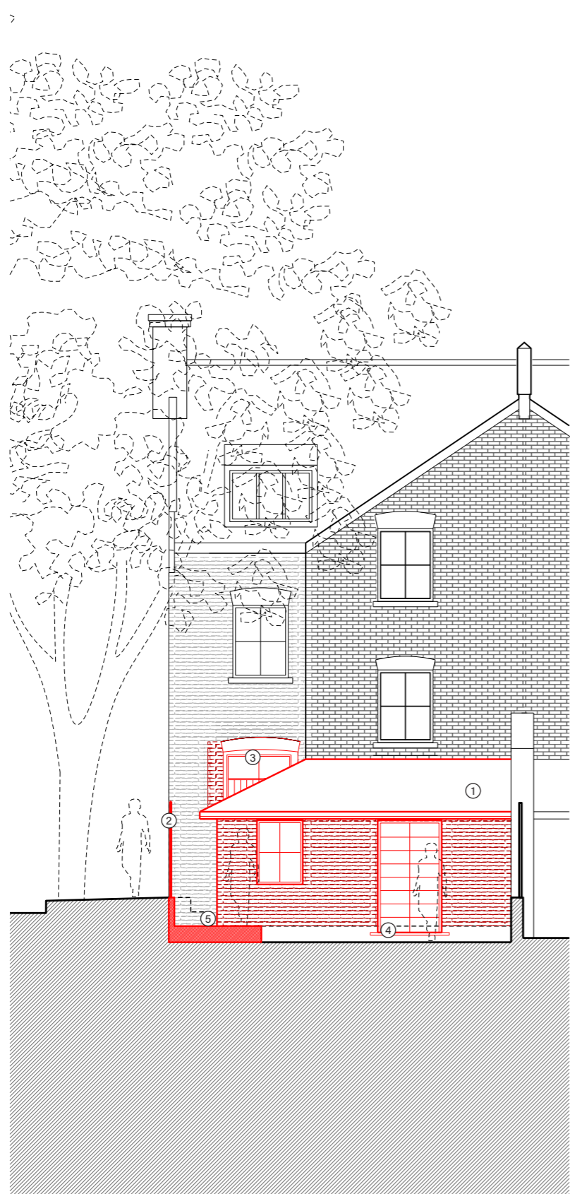
Existing/ Demolition Rear Elevation
