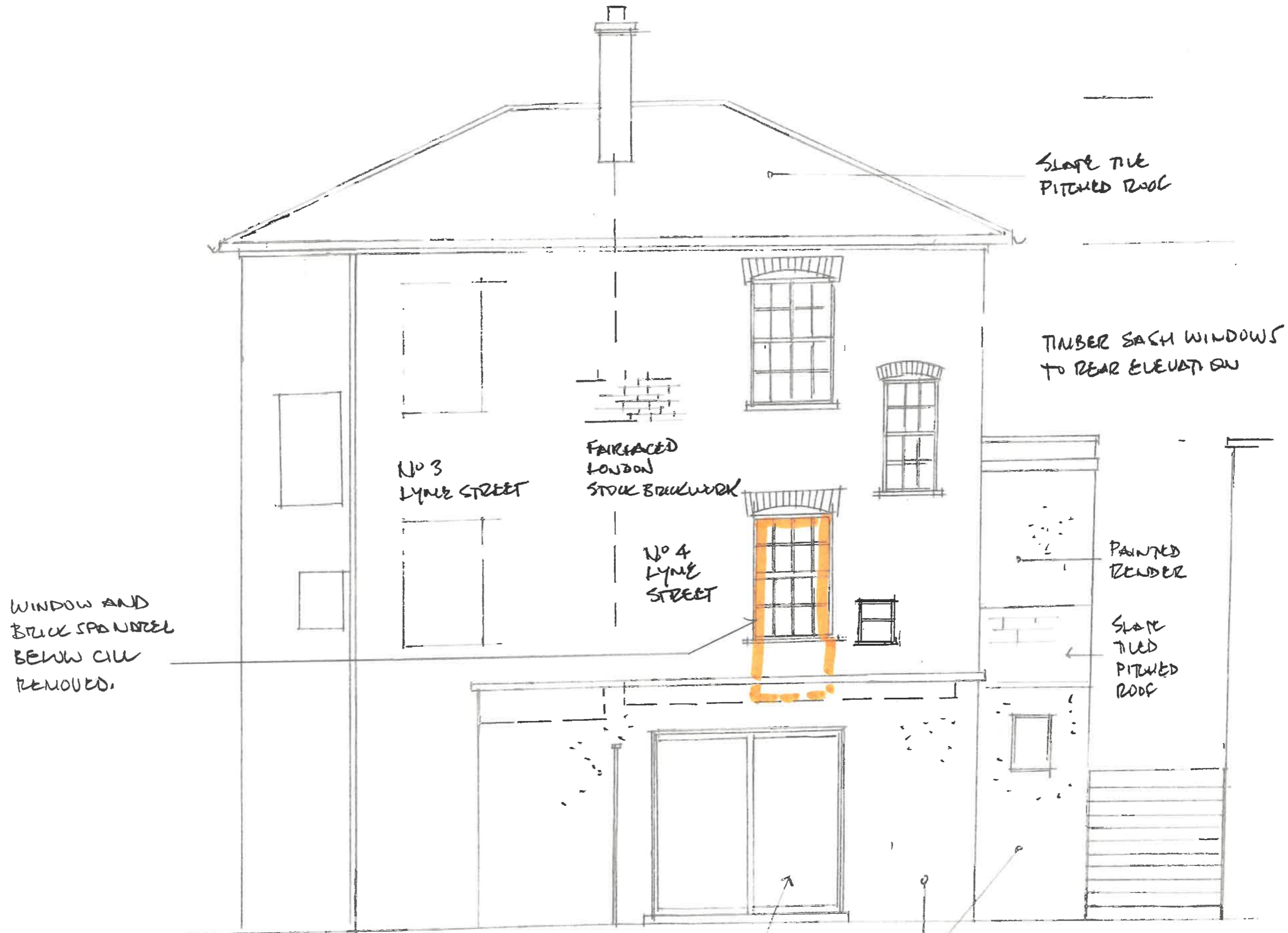
EXISTING REAR ELEVATION SHOWING DEMOLITION AREA
