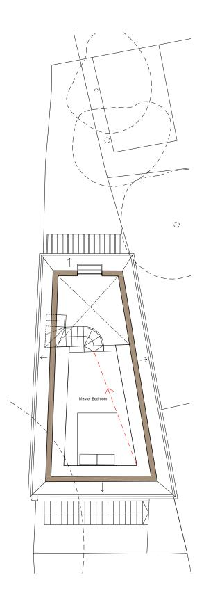
Egress Window 01 Opening sash window Openable area:  $1094x655mm = 0.72m^2$ Sill height from internal FFL: 812mm Vertical escape distance FFL to external ground: 3021mm
