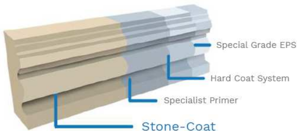
Figure 8 - Proposed custom-made stone coat moulding illustration by Built-Lite (UK) Ltd
