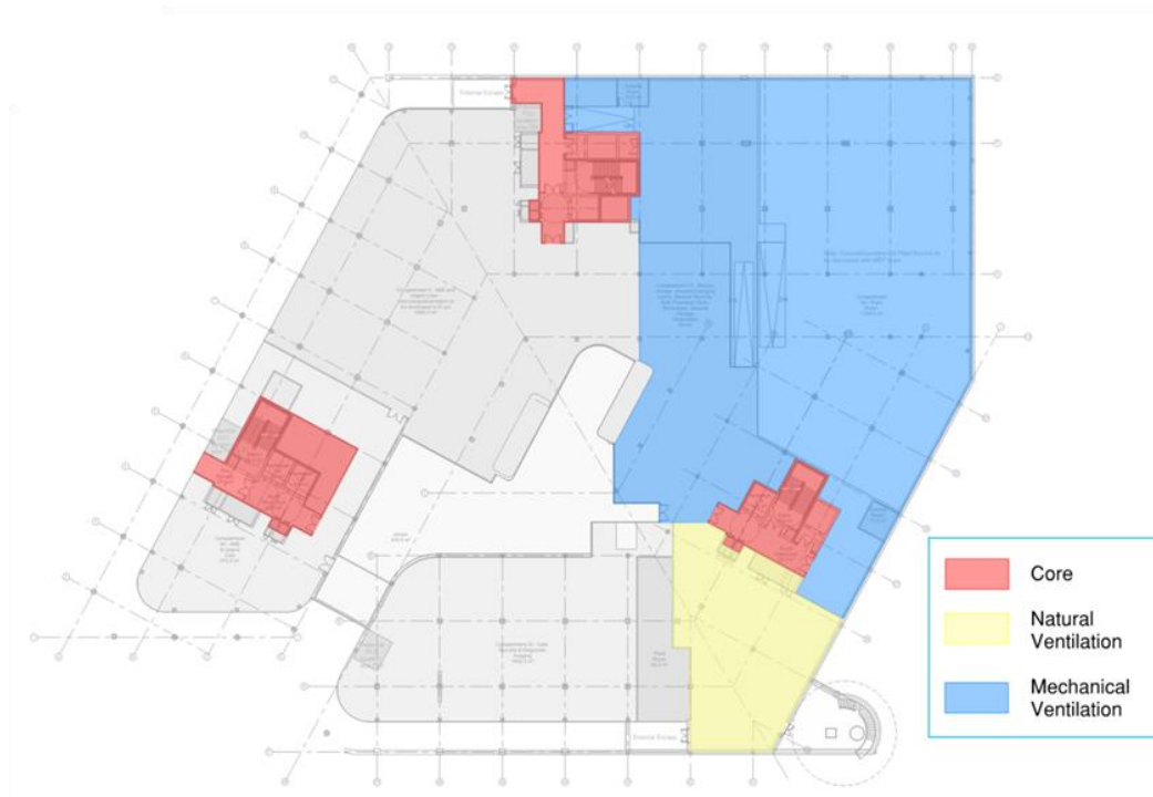
Figure 7-2: Configuration of lower ground floor ventilation
