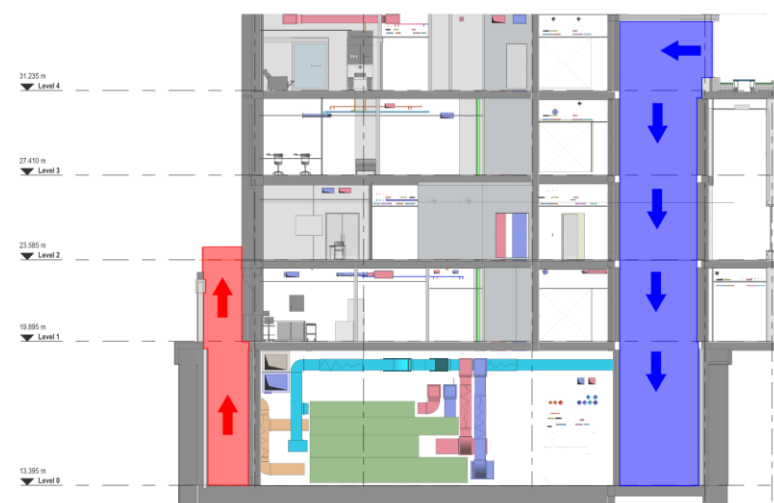
Figure 2: Level 0 Ventilation Intakes & Exhausts
