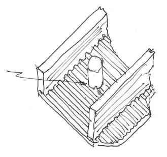
Cut laths where light removed to be removed carefully a plaster either side cut back
