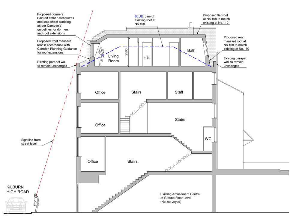
Proposed Section A-A (No. 108) Scale 1:100
