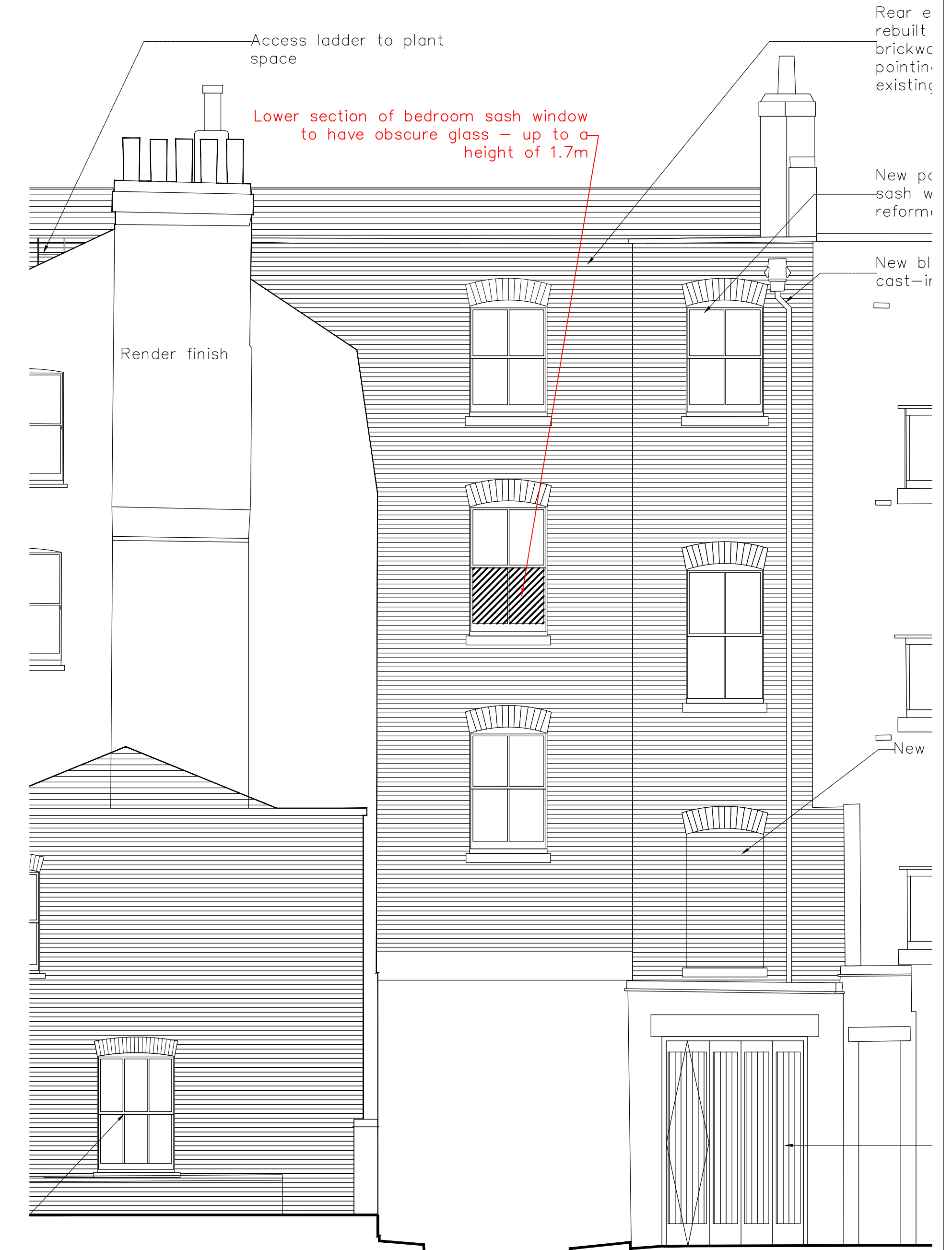
Rear Elevation As Approved Scale 1:50
