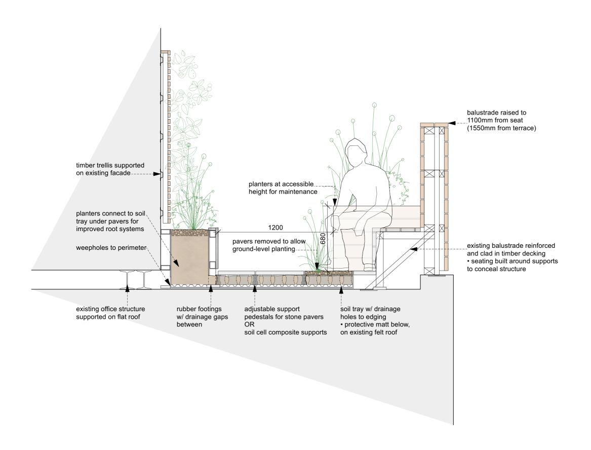
SECTION detail through main roof terrace showing planter, paving and bench construction
