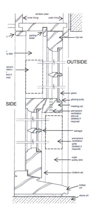
10 HILLTOP ROAD, LONDON, NW6 2PY Cross-Section through Old Timber Sash Window
