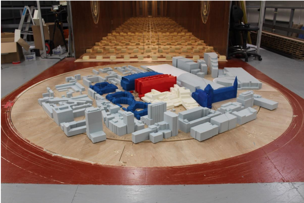
Figure 16: Photo of the model of the Proposed Development with existing surroundings in the wind tunnel (view looking north).
