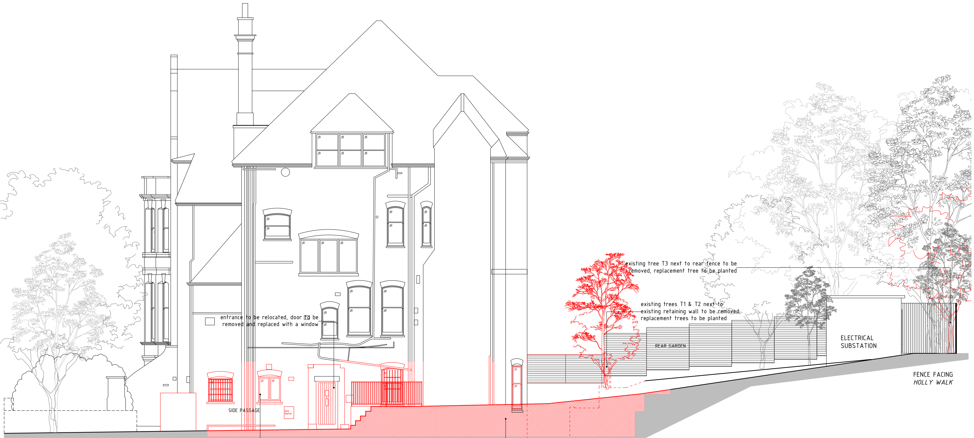
BOUNDARY WALL FACING FROGNAL GARDENS SIDE | SOUTH | ELEVATION - SECTION A-A existing side windows and sections of wall on lower ground floor to be removed providing structural support existing raised path to rear garden to be lowered to existing lower terrace level existing tree T3 next to rear fence to be removed, replacement tree to be planted existing trees T1 & T2 next to existing retaining wall to be removed, replacement trees to be planted REAR GARDEN ELECTRICAL SUBSTATION FENCE FACING HOLLY WALK
