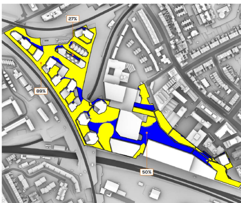
Figure 8. Plan by GIA showing areas of the new development that can receive two hours' sunlight on March 21 (in yellow) and those that cannot (in blue). North is at the top of the plan.
