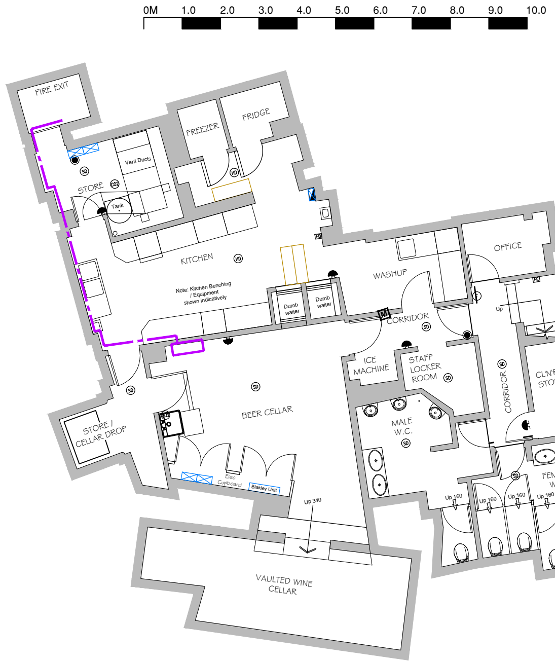
PROPOSED BASEMENT / CELLAR FLOOR PLAN - 1:100
