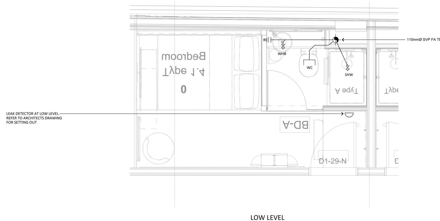
LEAK DETECTOR AT LOW LEVEL.
