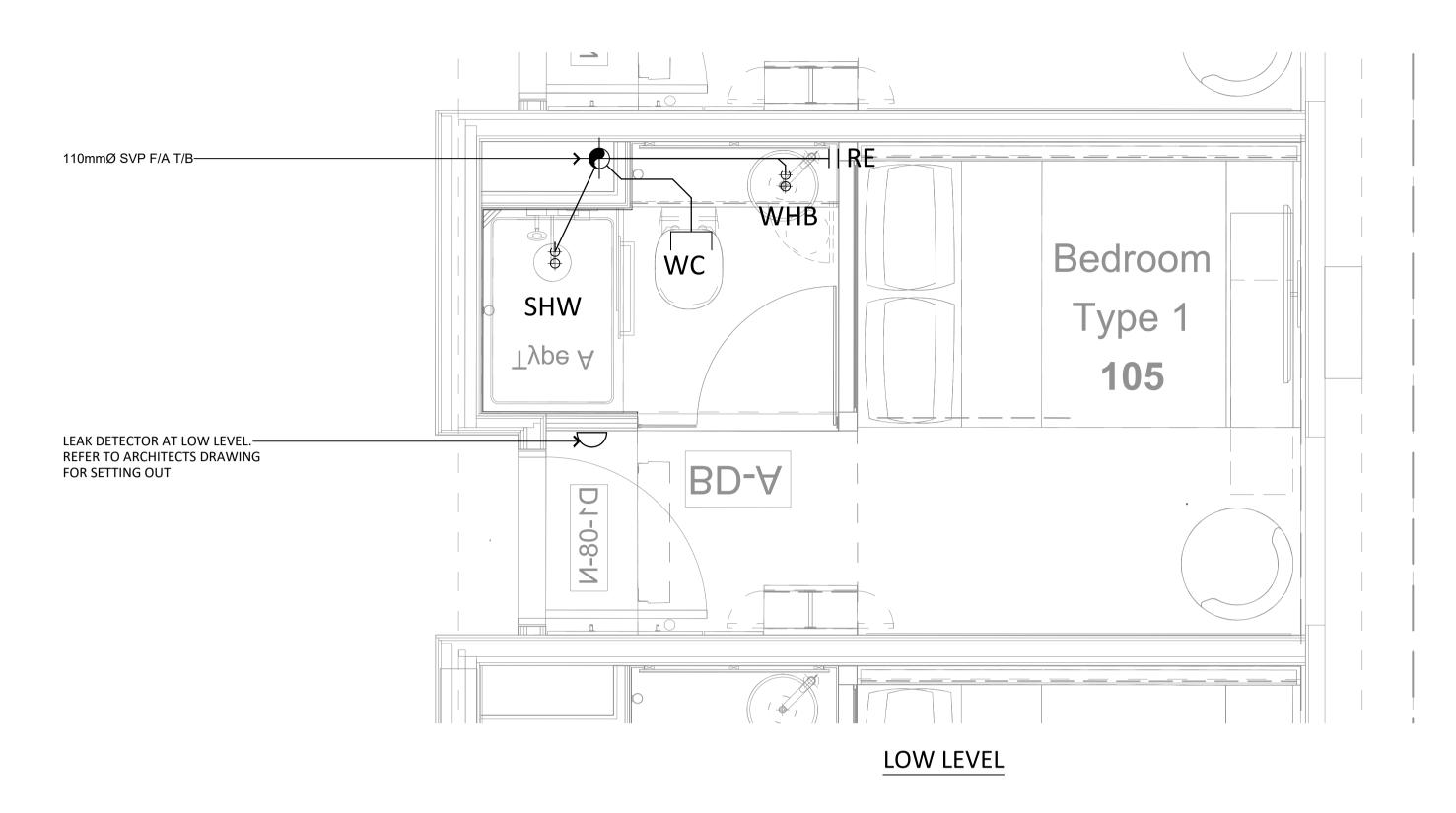
110mmØ SVP F/A T/B— DOMESTIC WATER SERVICES PIPEWORK-DROPS FROM H/L TO L/L FROM LEFT TO RIGHT 22Ø BCWS 22Ø DHWS F 15Ø DHWS R . . . ALL VALVES INSTALLED IN THE VERTICAL PIPEWORK ACCESS REQUIRED. EXTRACT AIR VALVE-DOMESTIC WATER SERVICES -PIPEWORK AT HIGH LEVEL \_ \_\_\_\_ \_ \_ \_ VRF FAN COIL UNIT TO BE MOUNTED -ABOVE THE DOOR
