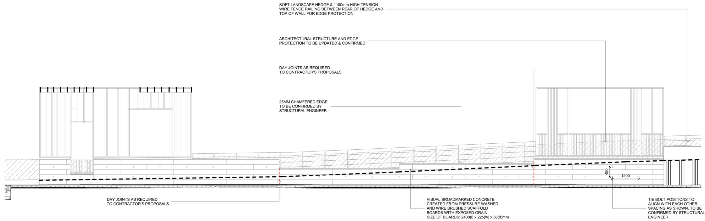
**ELEVATION 01: WT05 GARDEN WALL VISUAL CONCRETE SCAFFOLD BOARD BOARDMARKING**
