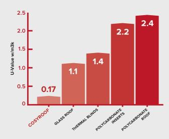
U value measures how well a building component heats the inside of a structure. The lower the U value, the less heat is lost.
