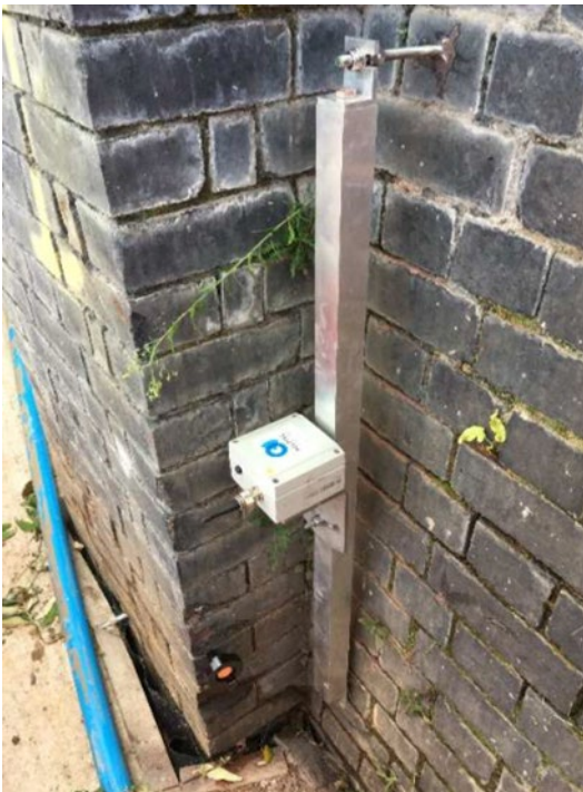
Figure 5 – Example of one metre tilt beam and a 3D prism.
