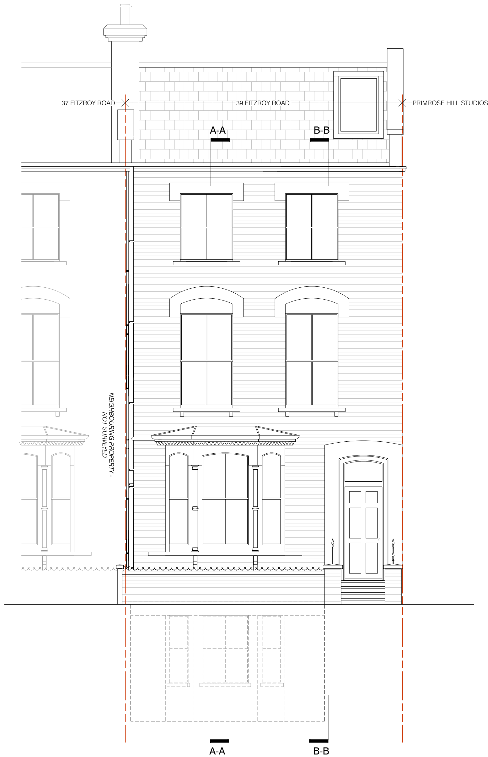
01 PROPOSED FRONT ELEVATION scale 1:50
