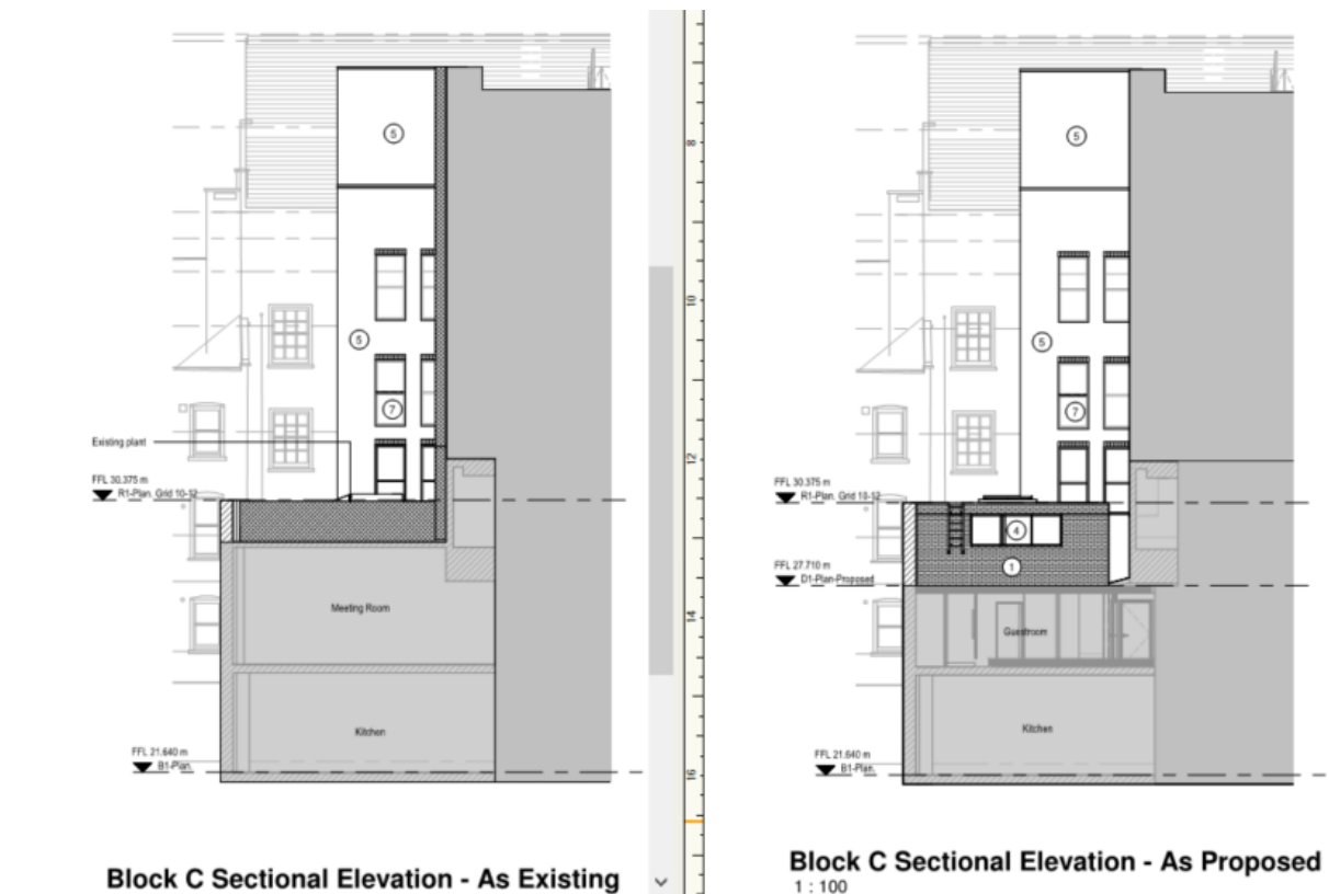
Figure 8: Existing (left) and proposed (right) section showing the height of the extension in relation to the existing parapet wall following removal of existing external plant.
