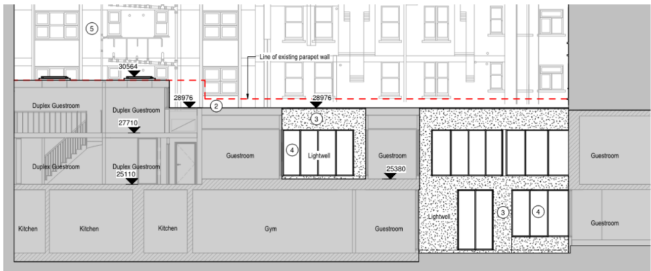
Figure 7: (Top) Existing section showing the plant, lantern rooflight and height of parapet wall (dotted in red) and (bottom) comparative proposed section showing the external works and height of parapet wall (dotted in red).
