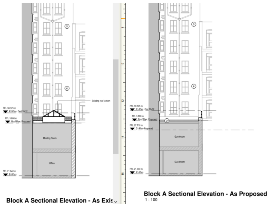
Figure 9: Existing (left) and proposed (right) section showing the works to the roof of the existing infill extension within the lightwell following removal of the existing roof lantern
