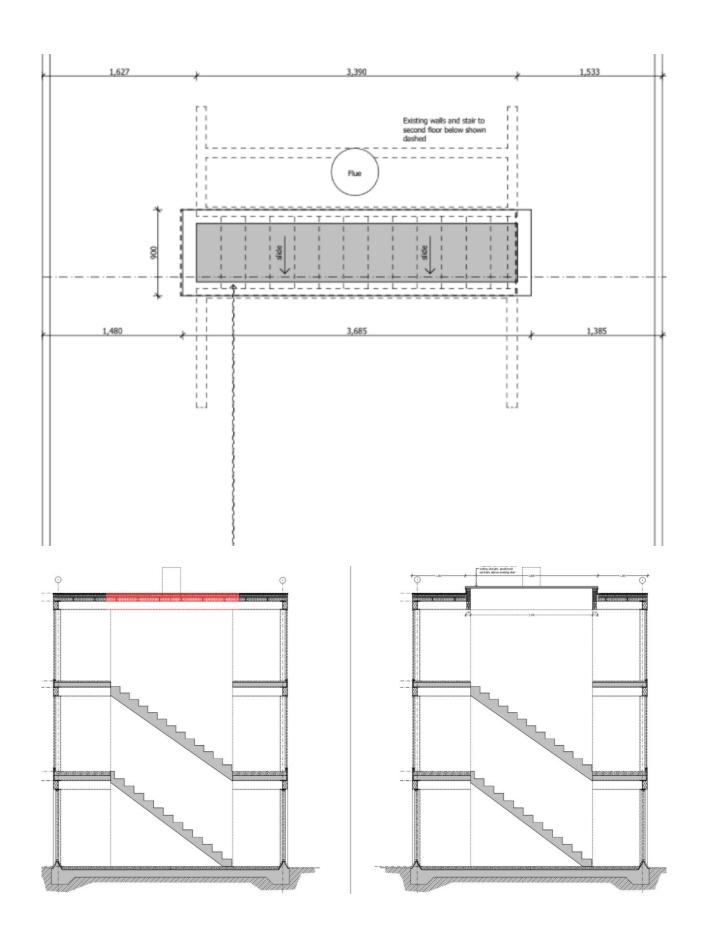
Proposed roof plan and demolition plan for the skylight above the staircase.
