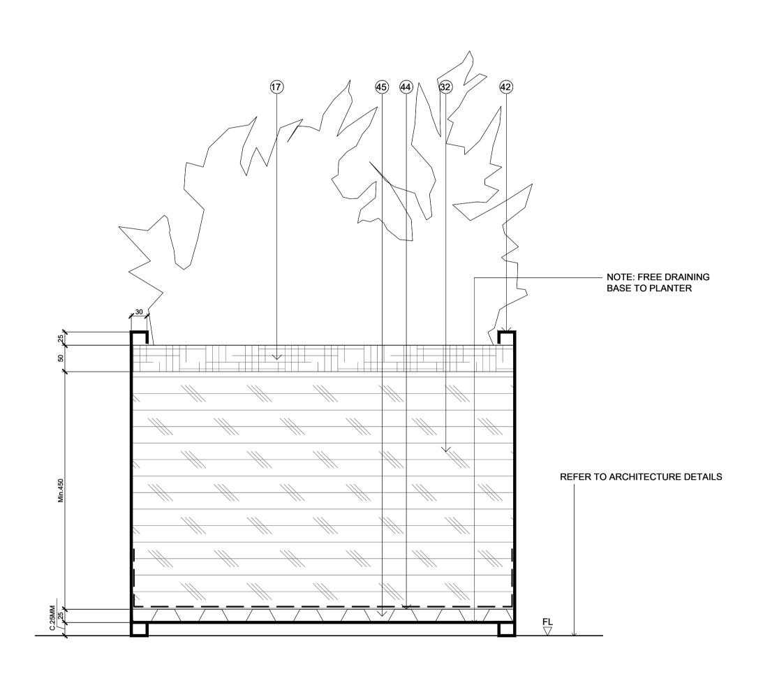
1 BESPOKE FREESTANDING METALWORK PLANTER TO PLOT I FOURTH FLOOR ROOF GARDEN: PLANTER TYPE PB3 SCALE 1:5
