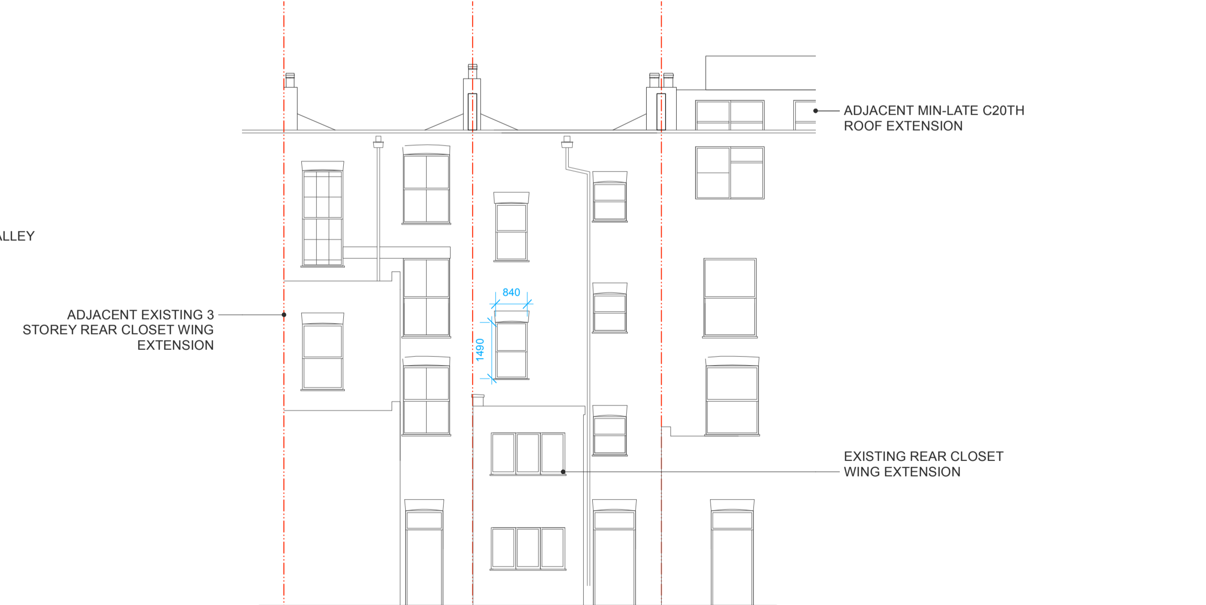
5 Rear Terrace Elevation 1:100
