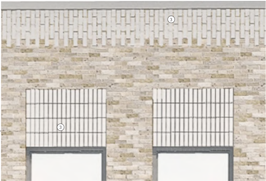
Brick parapet detail & Vertical stack bond Window Detail
