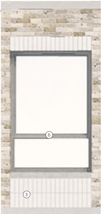
Aluminium window PPC coated frame with minimum 150mm reveal
