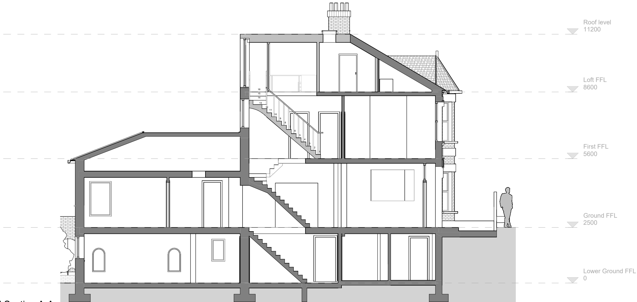
01 | Proposed Section A-A 1 : 100
