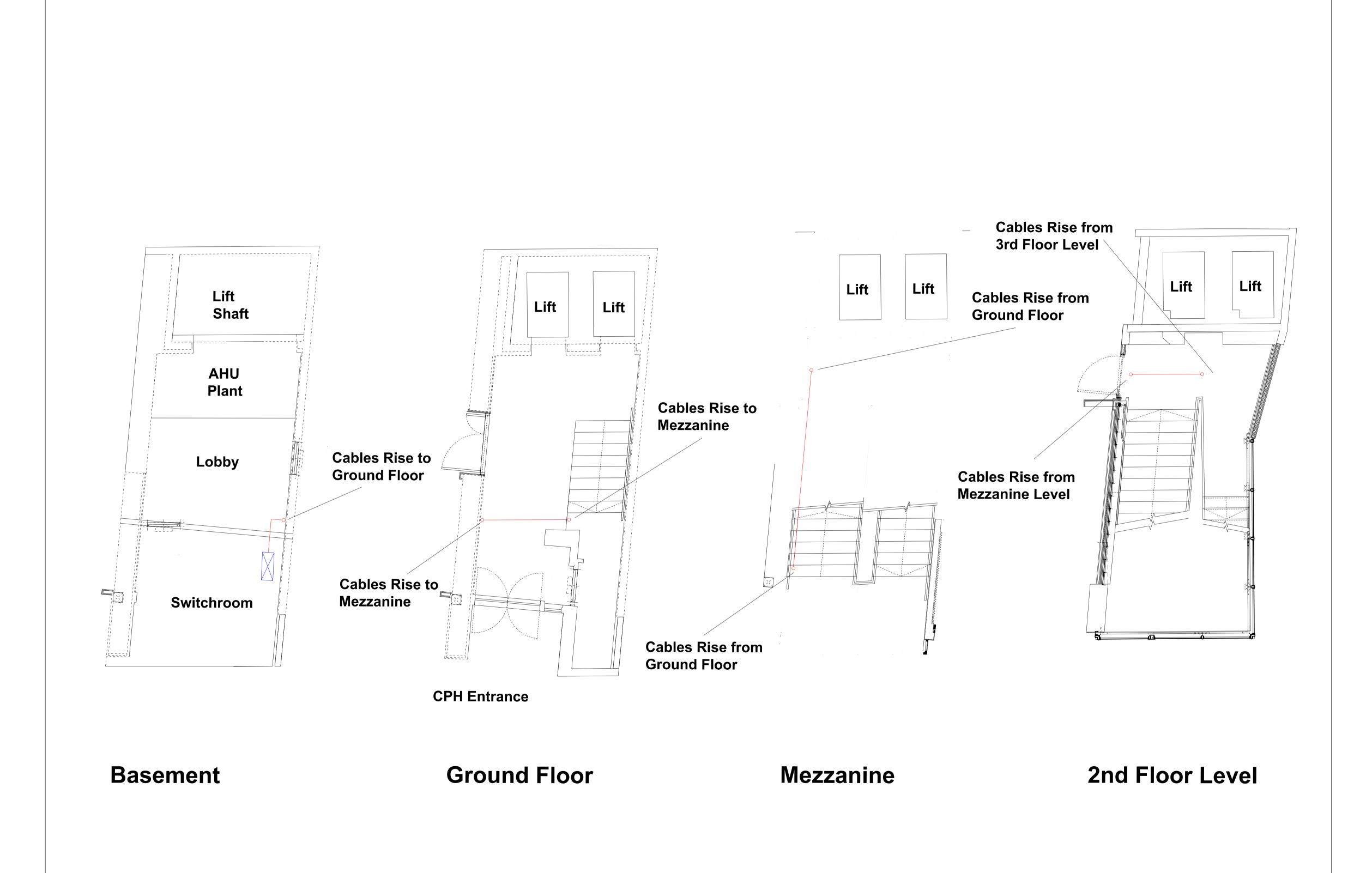
LEGEND New Sub- Main Fused Switches Proposed Route of New Sub- Main cables
