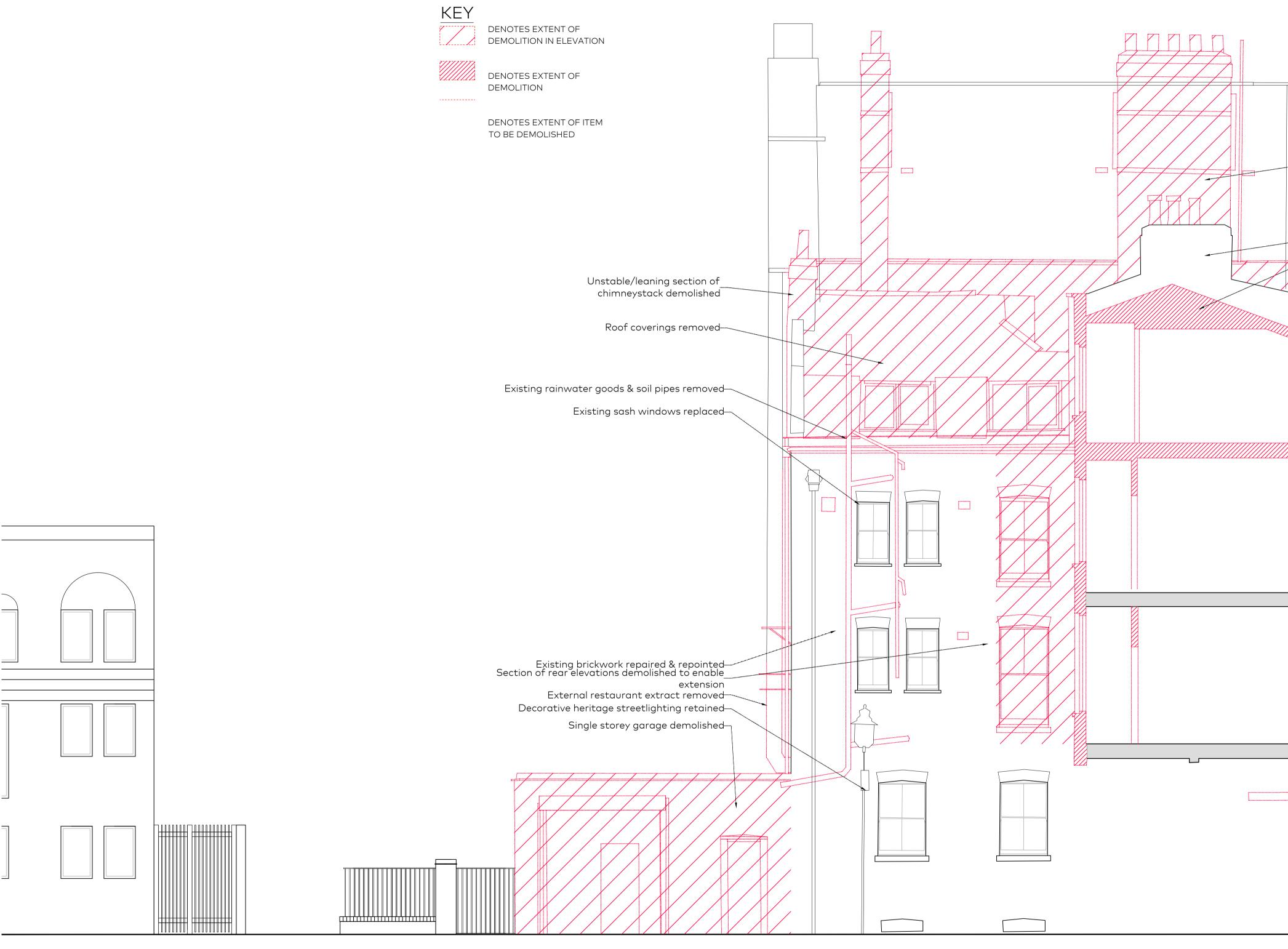
North Section AA, as existing with demolitions Scale 1:50
