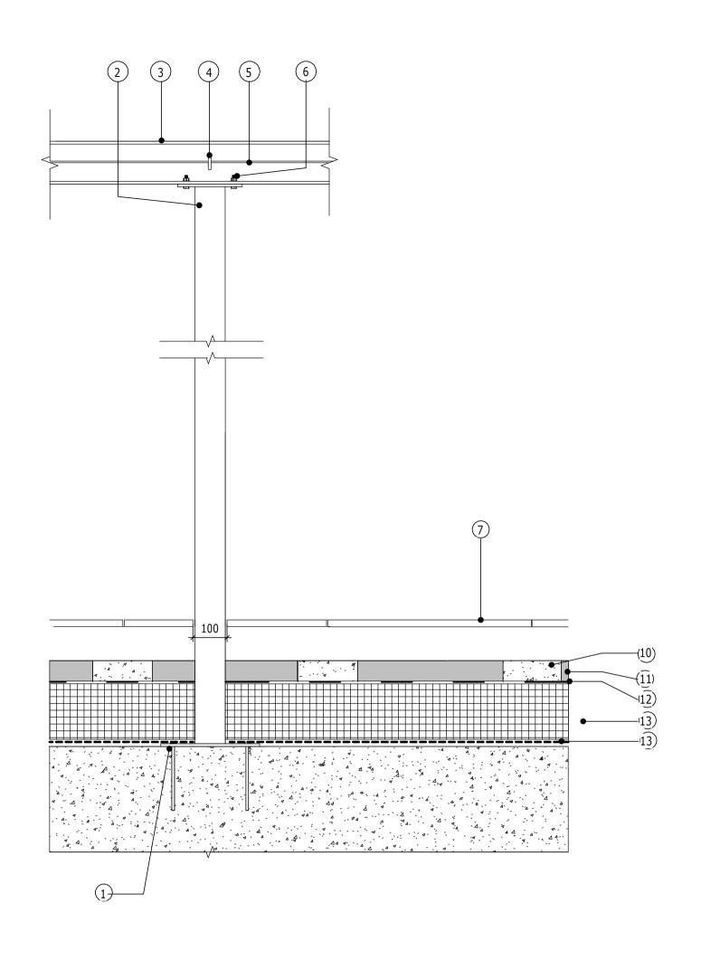
1. POST BASE PLATE & FASTENERS TO PERGOLA DESIGNER DESIGN AND SPECIFICATION, OVER SLAB AND WATERPROOFING.
