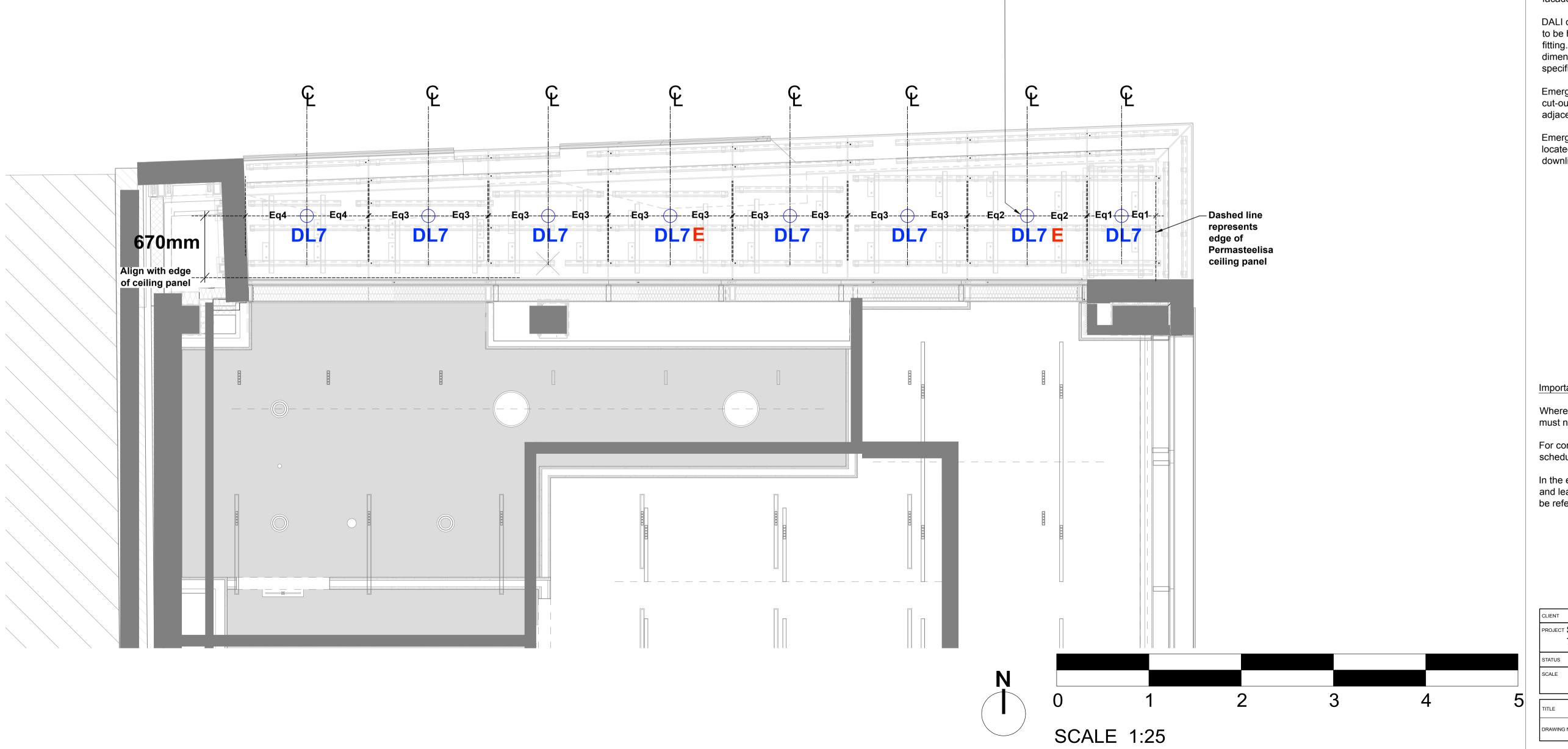
DL7- Downlight recessed into GFRC ceiling soffit to illuminate
