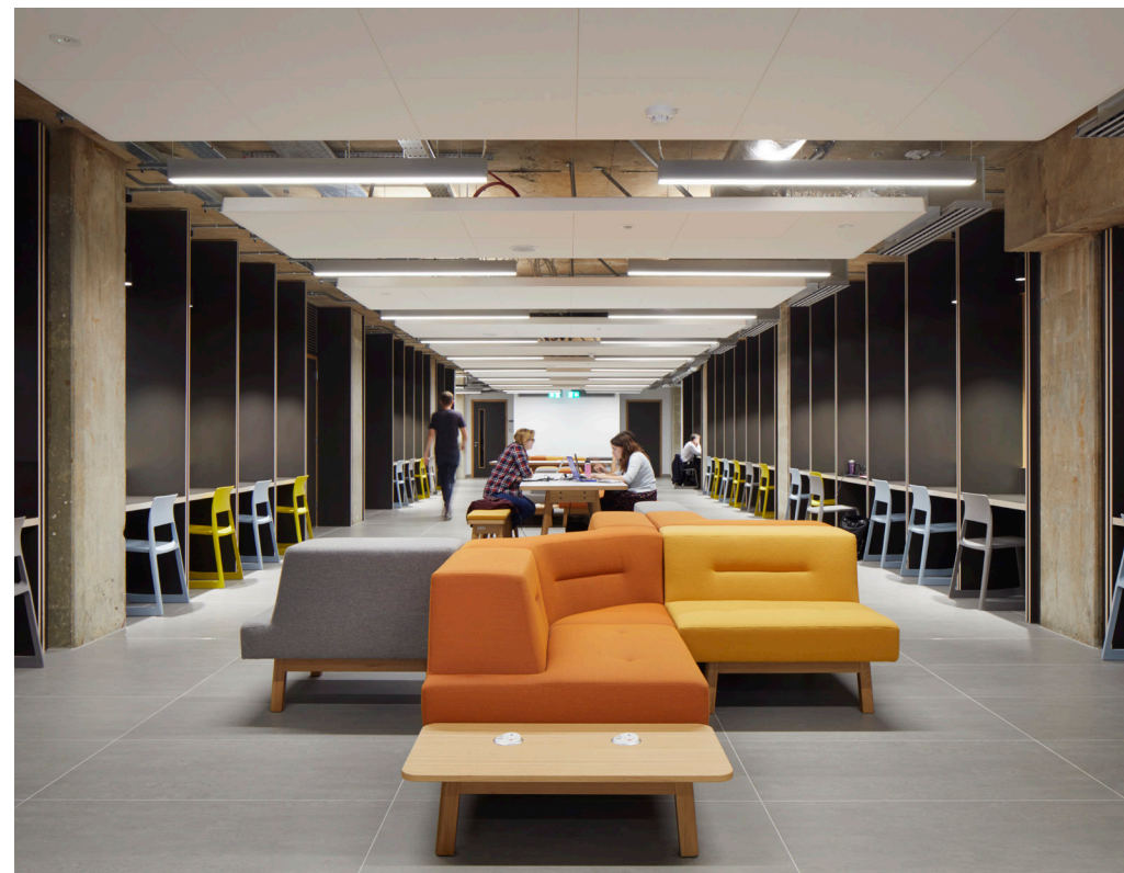
Typical details of laminate fins and exposed concrete soffits and acoustic rafts in Phase 1, Level 3
