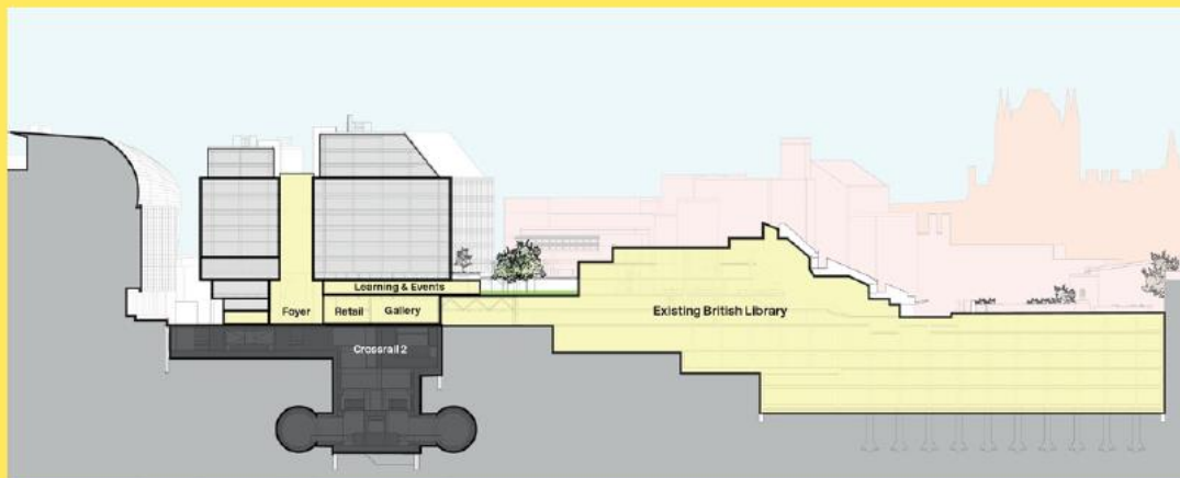
Cutaway of the proposed site and the Crossrail 2 works that will take place underneath
